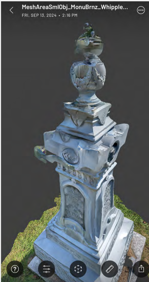
Fig. 10 (left): Mesh scan of zinc Whipple family monument; failure to render urn topper.
